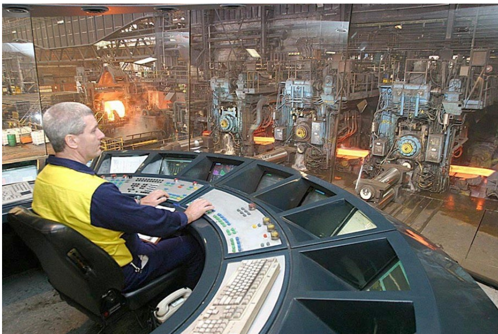
BlueScope Steel Port Kembla Hot Strip Mill finishing stands control room.
